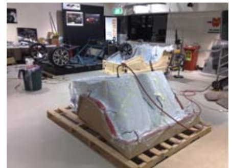
Figure 2: Carbon fibre fabric being laid-up onto FR-1 mould and vacuum bagged mould.
