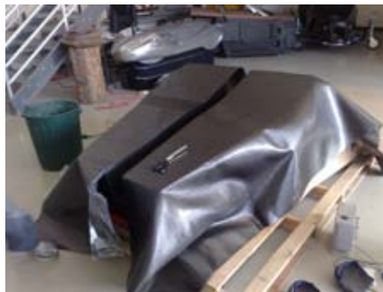
Figure 2: Carbon fibre fabric being laid-up onto FR-1 mould and vacuum bagged mould.
