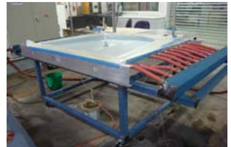
Picture of the manifold system designed and manufactured at Deakin University for the Quickstep fluid to flow through to heat the tooling and cure the part
